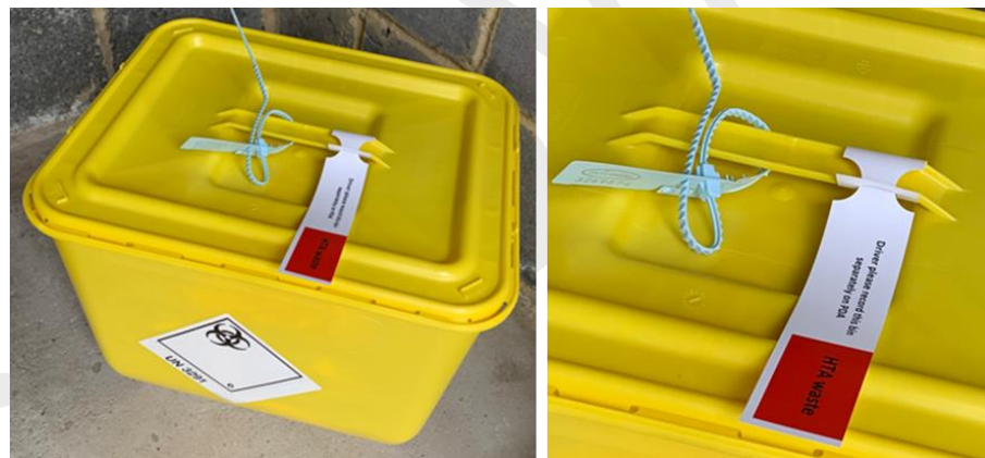
Figure 2: Yellow burn bin with blue waste tag and red HTA waste label required to request a certificate of destruction.
